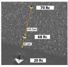
Properties such as hardness are developed within microns of the weld interface
