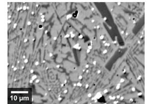
SHS9700E features a near nanoscale microstructure with grain sizes less than 400 nm
